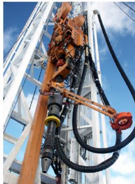
Figura 2 – Top Drive e internal casing drive.
